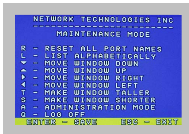
Figure 25- Maintenance Mode screen
